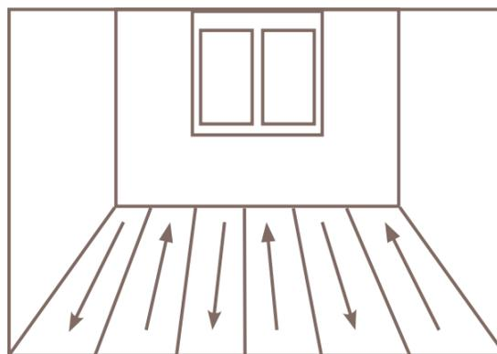
*2 - Tapisom plain: install the sheet in the same direction as the previous one installed.*
